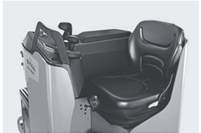
Suspended seat, adjustable to the weight of the driver for maximum comfort
