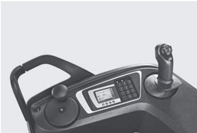
Steering wheel optionally on the left hand or right hand side
