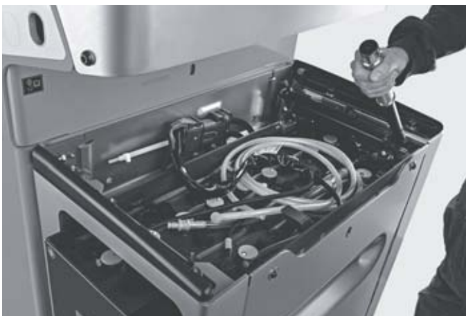
Battery change over the side as standard for highest availability and ergonomics
