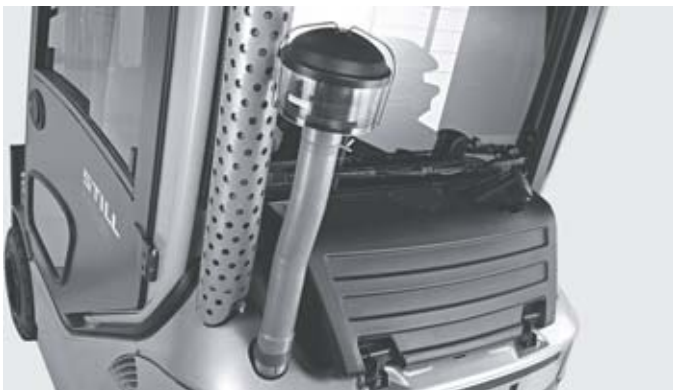
Cyclone air filter for clean engine air intake
